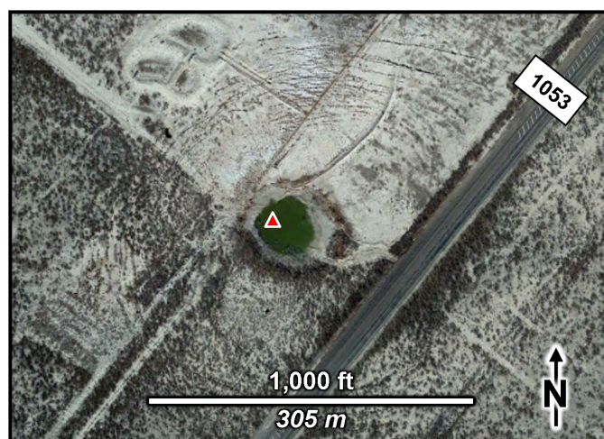
FIGURE 12. Concentric ground fractures extend at least 1000 ft (305 m) out from Site A subsidence feature adjacent to Farm-to-Market Road 1053. Pond at center of depression is about 180 ft (55 m) in diameter and covers about 0.5 acre (0.2 hectare). Location of repurposed Holladay well is shown by red triangle. Photo from Google Earth dated December 2019.
